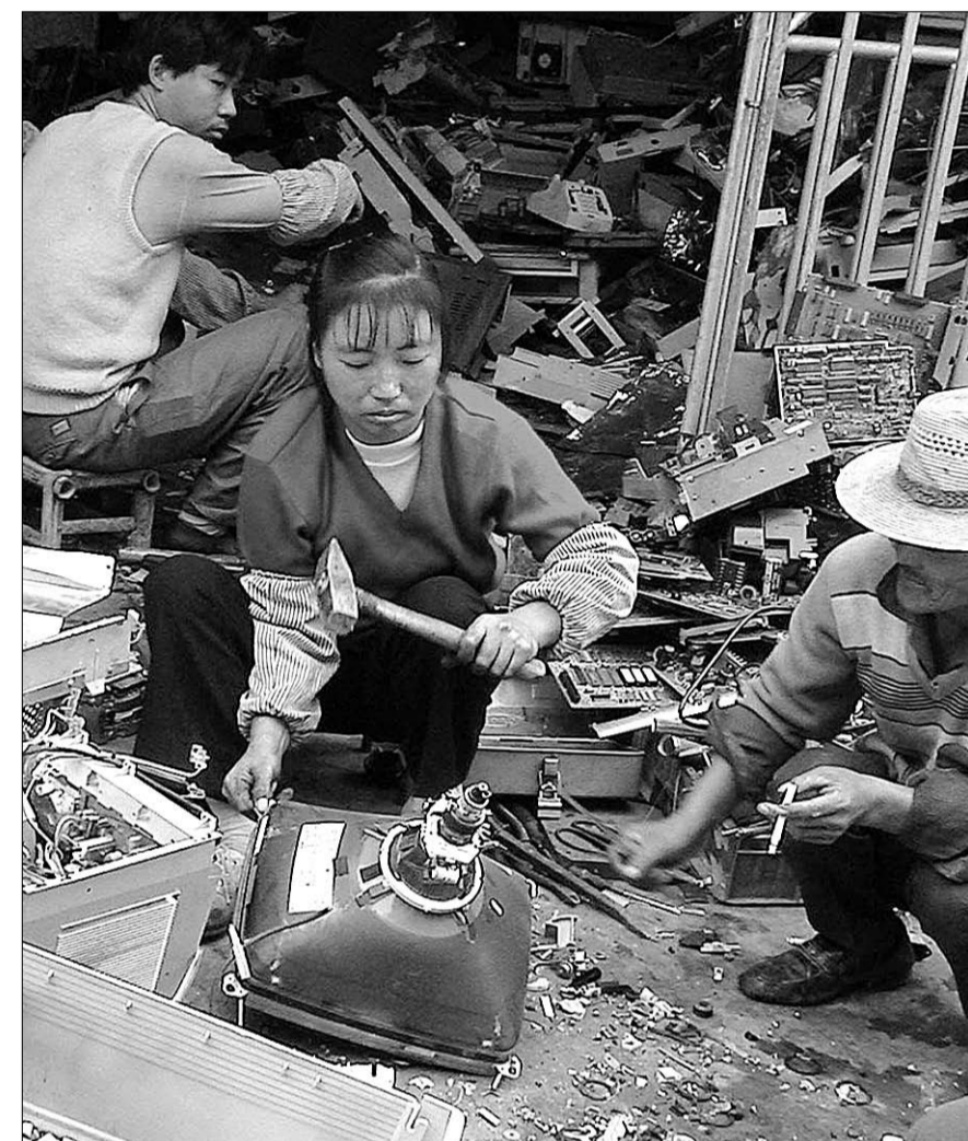
Woman in Guiyu smashes a cathode ray tube from a computer monitor in order to remove the copper laden yoke at the end of the funnel. Monitor glass contains lead but the biggest hazard is the inhalation of the highly toxic phosphor dust coating inside. The glass is later dumped in irrigation canals and along the river where it leaches lead into the groundwater. BASEL ACTION NETWORK 2006
